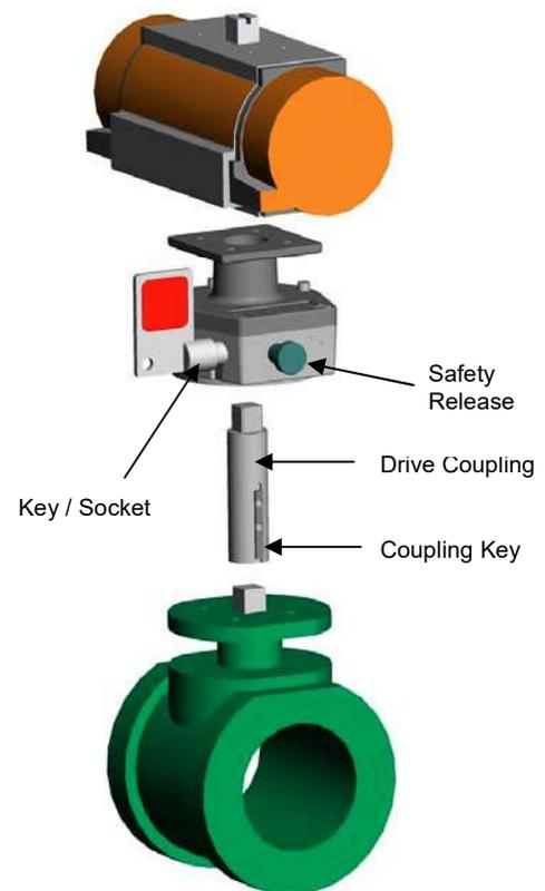
**IOM FOR DYNATORQUE D-STOP™ PARTIAL STROKE TESTING DEVICE (DS TYPE)**
