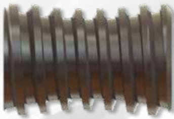
Single Start Standard Efficiency Worm Gear Inherently Self-Locking Less Than 35% Efficient
